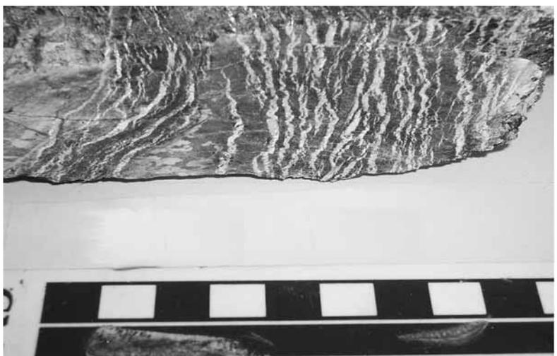
FIGURE 3. Cut slab of serpentinite from the Coolac Serpentinite, NSW, showing spaced array of asbestos veins up to 3 mm in thickness. Asbestos minerals (mainly chrysotile), comprise about 30% of the rock volume. Photo by Brenda Franklin.
