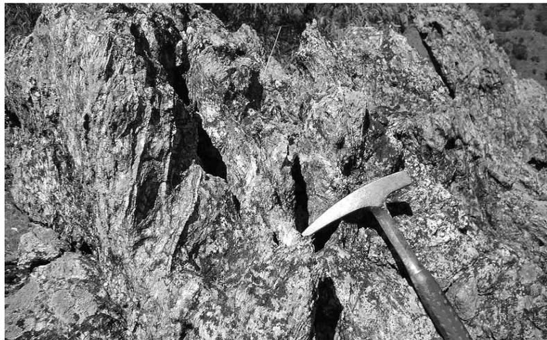
FIGURE 2. Outcrop of serpentinitised harzburgite from the Coolac Serpentinite, NSW, with approximately 10% cross-fibre veins of chrysotile asbestos.
